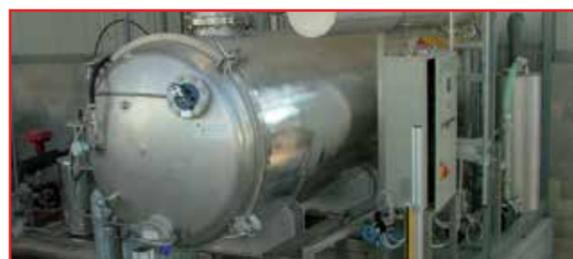
Using “clean” separation technology, EVALED evaporators offer a complete solution to surface treatments waste water.
